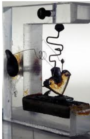
The first transistor (1947)
